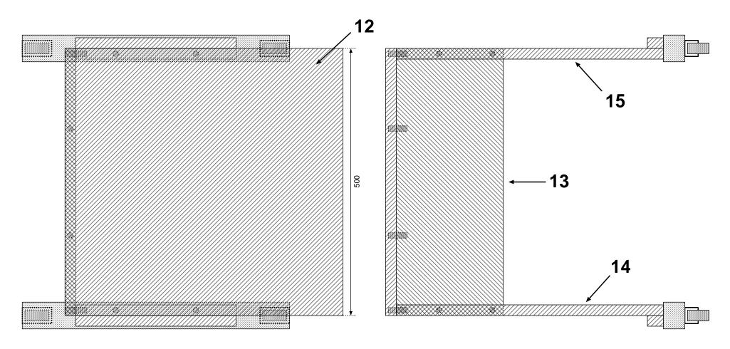
The wheels are attached to a spruce beam of ca. 3x4x50 cm. which was glued onto parts 14 and 15. A 30 cm. piece of leftover MDF was used to secure the attachment. Otherwise more 8 mm. dowels used in the butt ends of the boards.
